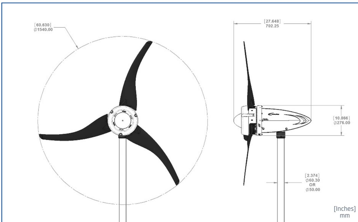
The LE-600 has a design life of 20 years, but due to its modular design and ease of maintenance, the turbine could easily run indefinitely.
